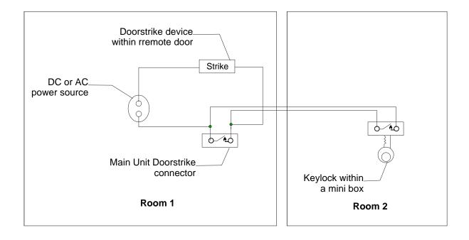
Fig 4.- Door access control from phones and a dedicated keylock installed in a separate area. (The keylock can rather be a simple switch.)
