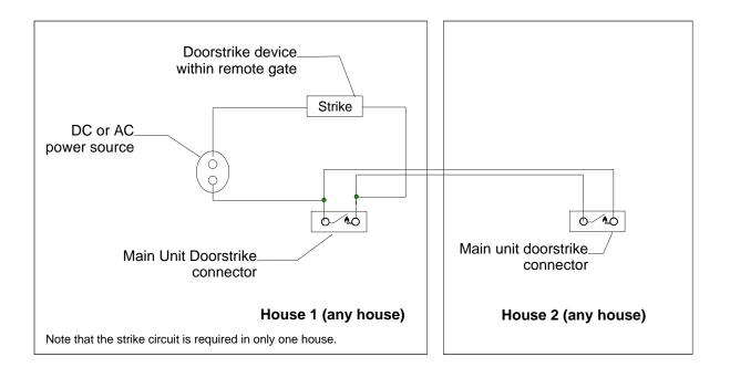
Fig 3.- Common gate control from two contiguous houses (This setup applies even if your neighbor has a different phone system. It does not matter which system manages the strike circuit.)
